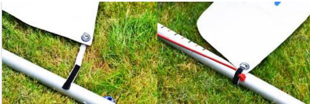
Attach the clew strap, pull it all the way thru the clew as shown, then pull the end through the ring and fasten in to place around the inhaul elastic. Do this closer to the boom cleat so there is a low amount of tension on the inhaul elastic. Its easier to rig the boom on the ground especially in breezy conditions. You can also leave the sail on the ground until you're ready to go sailing, this reduces unecessary wear.
