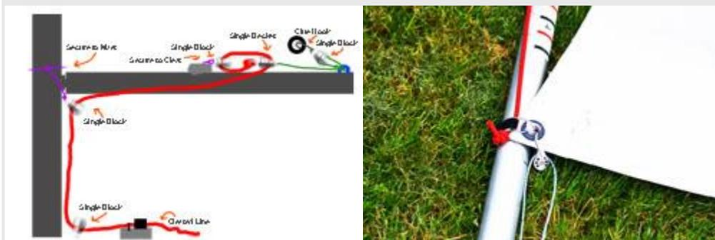
Using a clew hook makes it easy to clip on the outhaul, the outhaul should be clipped on after the inhaul and clew strap are fastened. The knots used are bowlines tied as small as possible. You can also get splice the ends to create less friction on the lines. The best blocks are ball bearing with a reinforced plastic shell. The plastic reduces friction when the blocks are tensioned off angle. The plastic can eventually get worn down so inspect them periodically.
