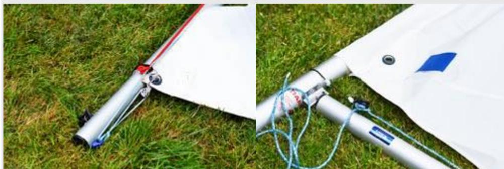
Tie the end of the non-cleated line to the boom fairlead. Its important to use a strong and thin line for this to reduce friction. Tie a false knot to keep the outhaul intact while stepping the mast. To do this create a loop, then instead of pulling the end of the line through, create another loop and pull the second loop tight, if you've tied it succesfully when you pull on the end of the line the knot will come undone simply by pulling. *Continued...*
