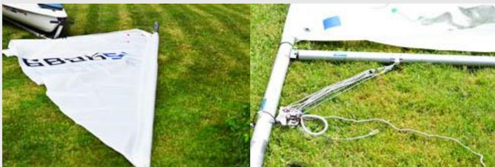
Slide the sail sleeve over the mast keeping the sail lined up with the goosneck (part where the boom attaches) Attach the boom to the goosneck and clip in the boom vang. It's important to put a piece of rigging tape around the boom to keep the vang key from slipping out downwind. The boom can come off if the vang detaches while sailing. *Continued...*
