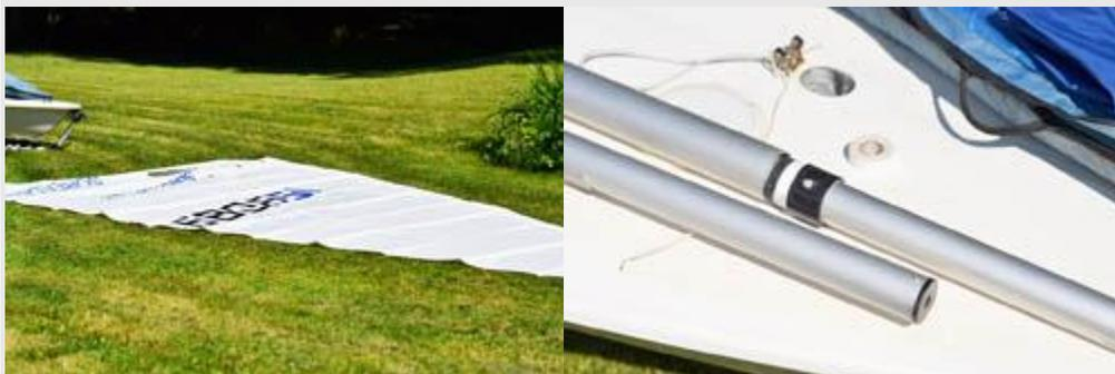
Lay the sail out flat then, put the upper mast and lower mast together (the upper mast and boom are the same for Std, Radial and 4.7 rigs) it is a good idea to wrap a piece of rigging tape around the top of the upper mast as shown. This ensures a tight fit and keeps the luff of the sail in the proper position. (Visually inspect the spars for damage and defects)
